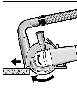
Switch on the machine and place the front part of the cutting guide on the workpiece. Slide the machine with moderate feed, adapted to the material to be worked.
