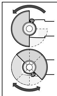
Place the protection guard **6** on the spindle collar. Adjust the position of the protection guard **6** to the requirements of the operation. Lock the protection guard **6** by tightening the locking screw **5** using a Phillips screwdriver.
